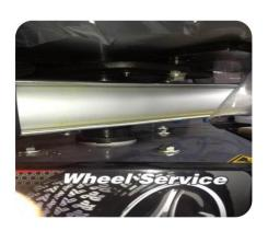
Turntable Cylinder 360kg maximum clamping power
