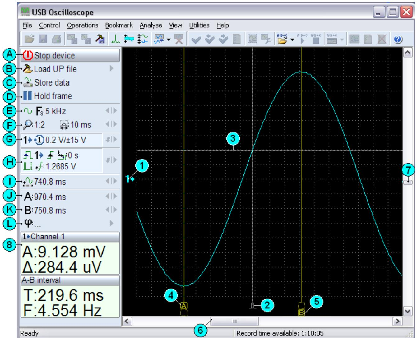
fig. 4. Program window in analogue oscilloscope mode
