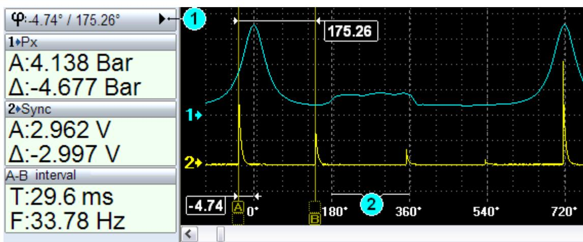
fig. 20. Phase measurement.
