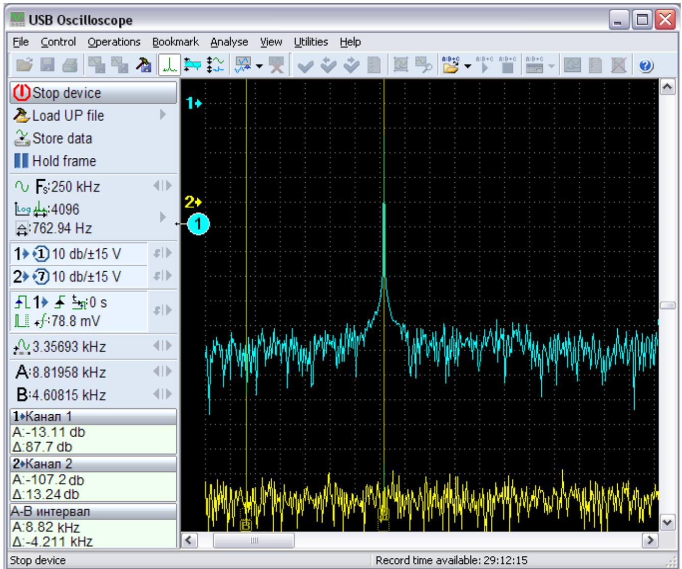
Fig. 8. Program window in spectrum mode
