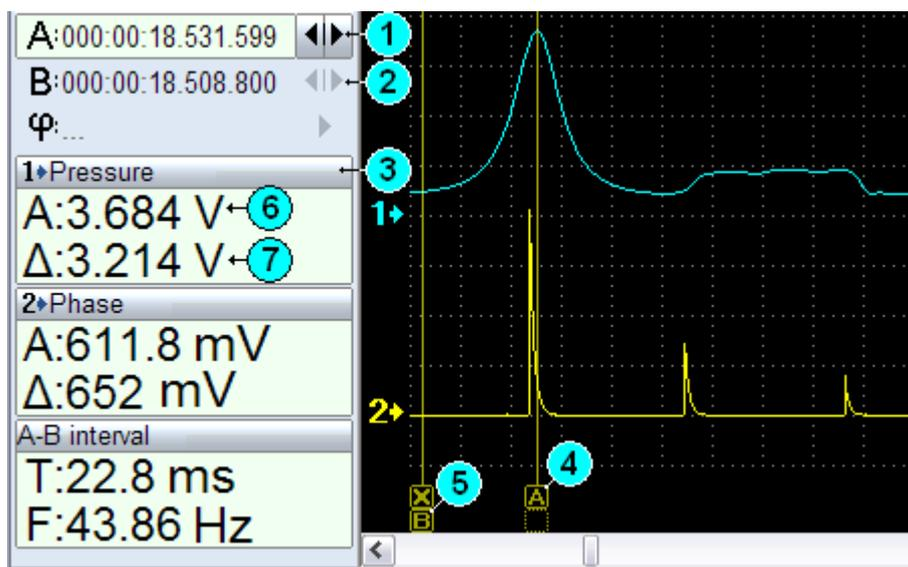
fig. 19. Measurement panel and A and B markers.
