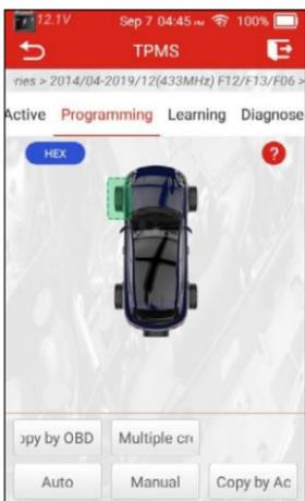
4. Place a LAUNCH-sensor close to the TPMS antenna of the tool, select the desired wheel position and tap **Copy by OBD**.
