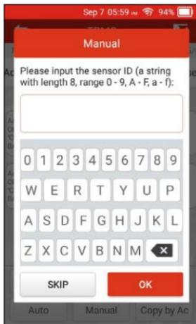
Use the on-screen virtual keypad to input a random or original (if available) sensor ID and tap **OK**.
