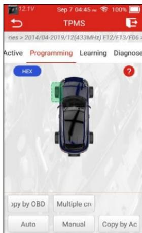
Select the specific wheel position and tap **Copy by Activation** to retrieve the information of the original sensor. After the information is retrieved, it will be displayed on the screen.
