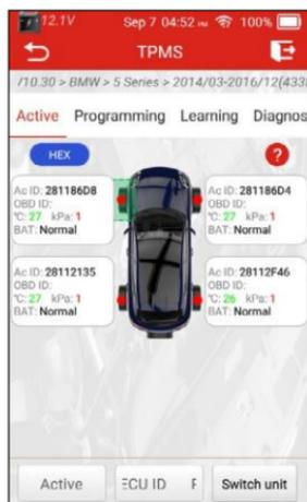
If the users intend to read the original sensor ID stored in the ECU, connect the tool to the vehicle's DLC via the diagnostic cable and tap **Read ECU ID** to read the information of the four TPMS sensors. After the sensor information is successfully decoded, tap **OK**, it will be displayed in the *OBD ID* field.
