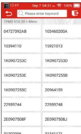
Check the original manufacturer number on the body of the sensor, and tap the corresponding OE number on the screen to enter the following screen.
