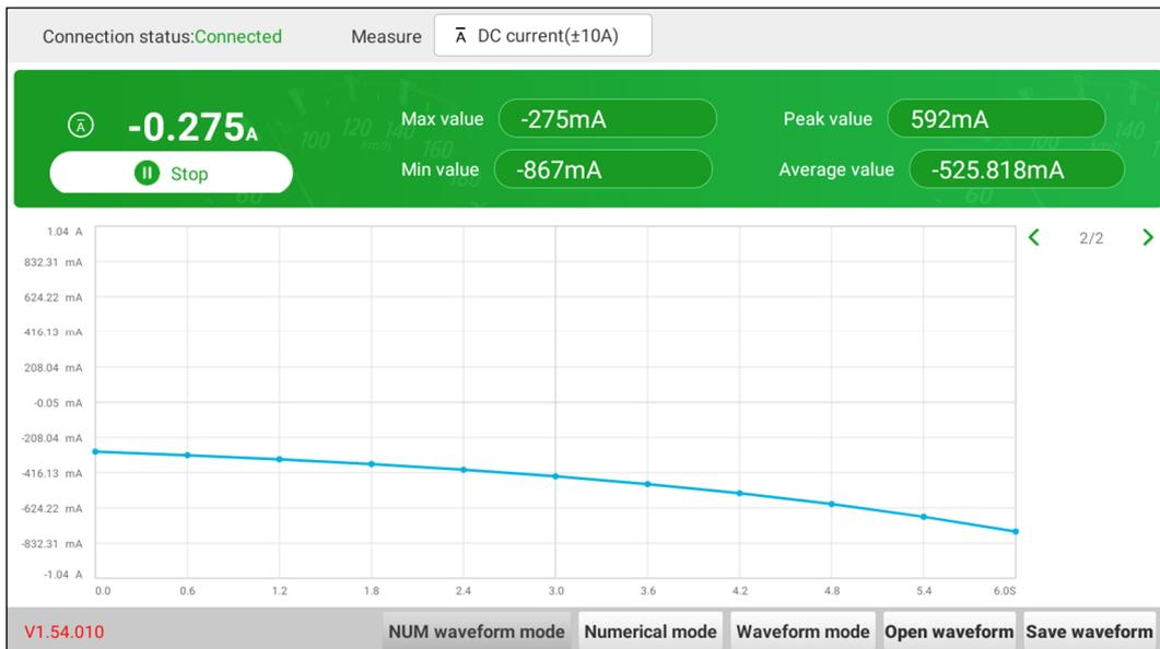
2. Select **DC current/AC current** and corresponding range. Tap **Not connected** to search for EM101N. When it is successfully connected, the diagnostic tool will display connection status.
