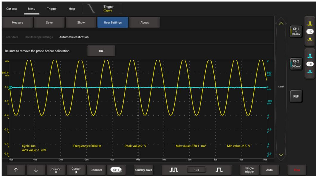
Tap **OK** on the pop-up message box to start calibration. The LED on the EM101N starts flashing and the prompt message “Calibrating, please wait” will appear on the upper left corner of the screen.
