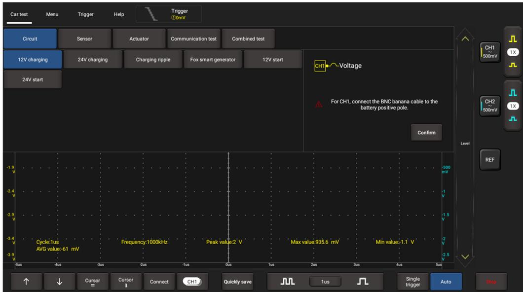
Tap to select the desired automotive part, the system will automatically configure the option to the preset parameters. The user does not need to make any settings. Just follow the on-screen instructions to make connections and proceed.
