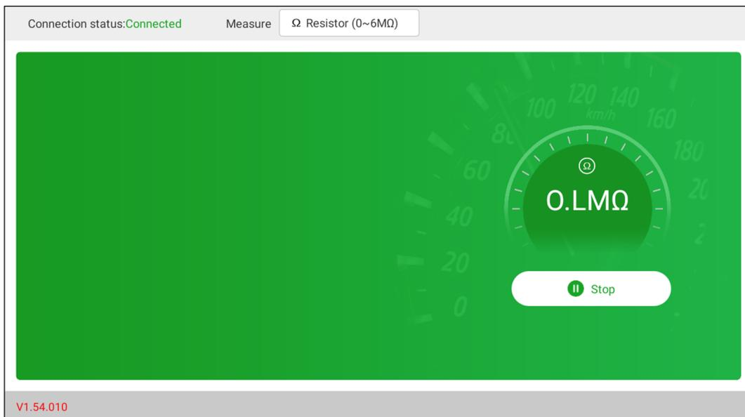
2. Select **Resistance**, tap **Not connected** to search for EM101N. When it is successfully connected, the diagnostic tool will display connection status.
