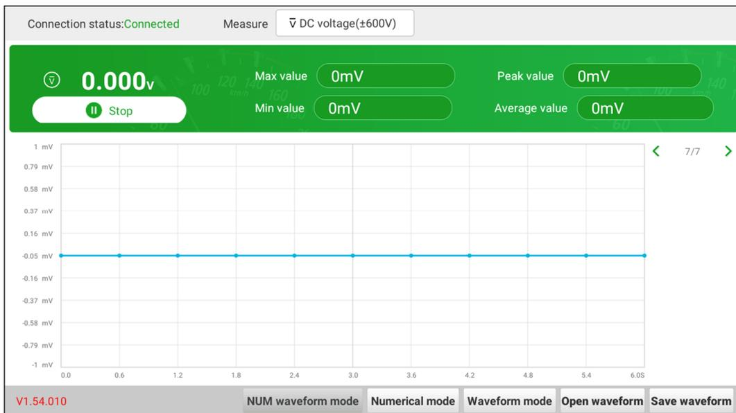
2. Select **DC voltage/AC voltage** and corresponding range. Tap **Not connected** to search for EM101N. When it is successfully connected, the diagnostic tool will display connection status.
