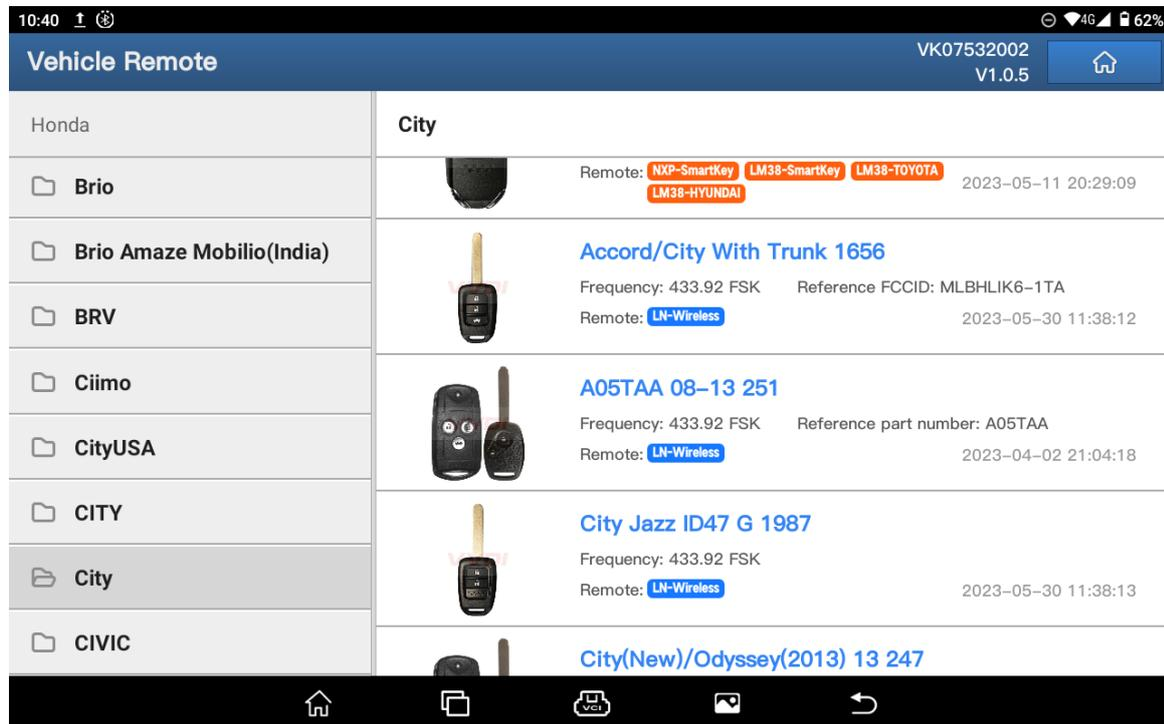
2. Place the electronic remote key in the key programmer to generate.
