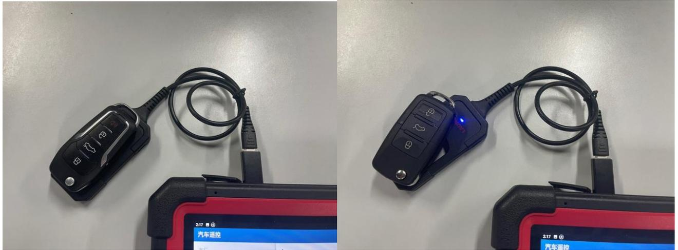
3. After the remote control is successfully generated, enter the [Set type of super chip] menu to generate the corresponding key chip.
