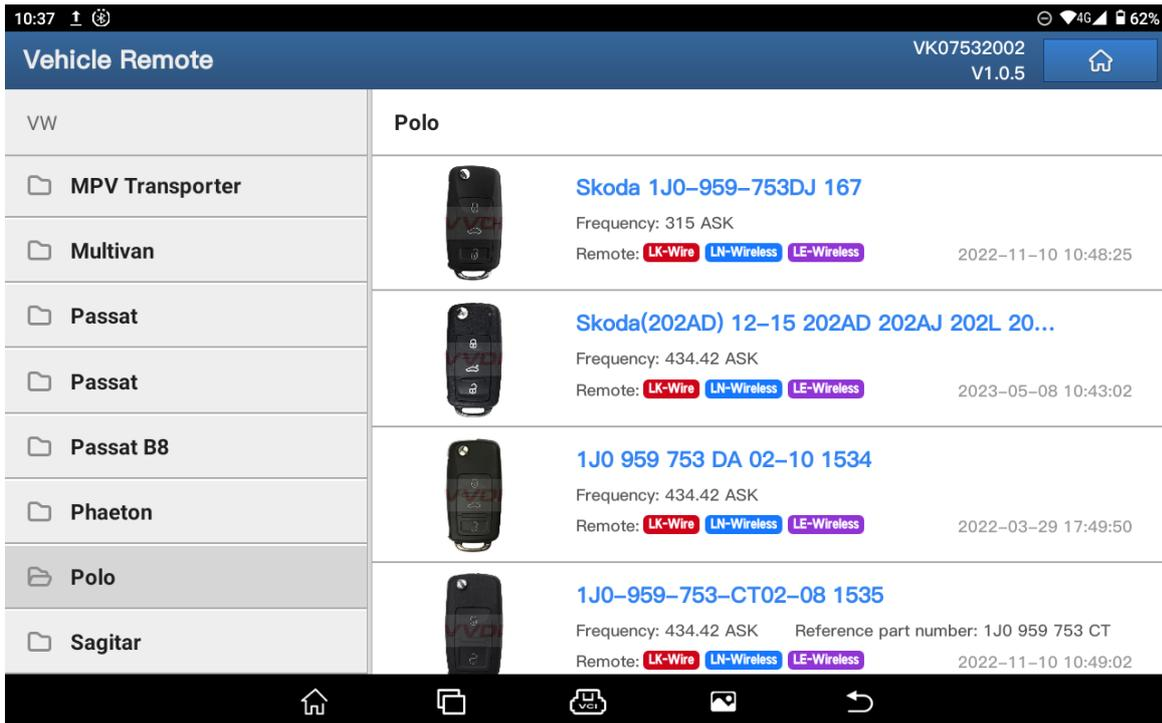
2. Select the corresponding key and place the super remote key in the key programmer to generate.
