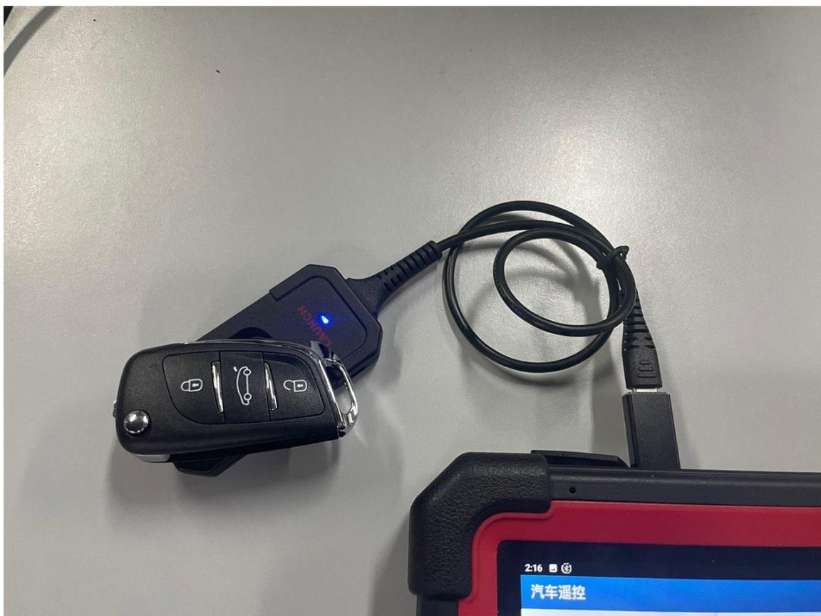
2. For car models without electronic keys, enter [Set type of wireless remote] to generate the corresponding key.
